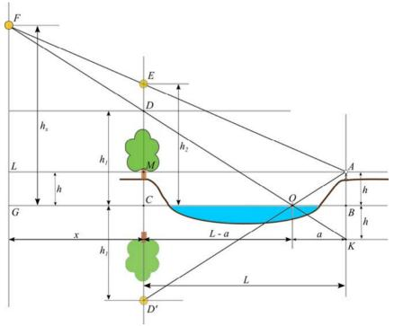
**FIGURE 2.** The scheme of paths of rays at taking of a photograph of a shining object, reflecting in water.
