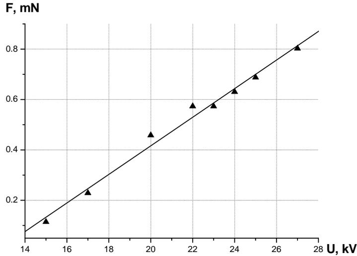
**FIGURE 2b.** Dependence of the force, acting on a ball with five needles, on its potential.
