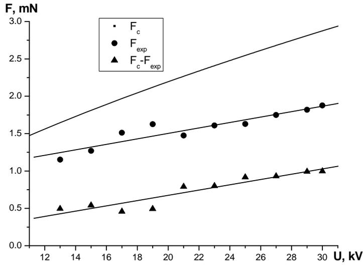
**FIGURE 2.** Dependence on voltage of a force, pushing away two plastic balls of diameter 4 cm.
