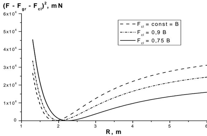
**FIGURE 3.** Dependence of a square of the forces sum  $F_s^2 = (F_c - F_{gr} - F_{cl})^2$  on a distance  $R$  between two BLs with a charge of everyone  $Q = 10^{-3}$  C. Function  $F_{cl}(R_{cl})$  is considered a constant.
