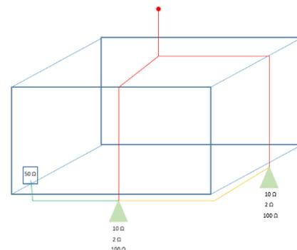
Dangerous secondary sparks can appear between the down-conductors and conductive parts around. The length of the spark that can be created depends of the lightning current, of the distance between the two electrodes and of the earthing system resistance value.
