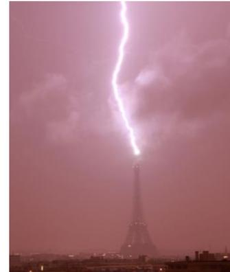
According to theory and to the distribution of the lightning current, the impact at the top can be estimated above 50kA.
