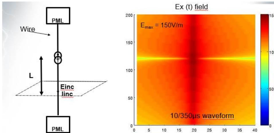
PML are Perfect Matched Layer. They enable to simulate an infinite volume of calculation in the FDTD method. It means that there is no reflection of the edge of the calculation volume.
