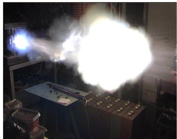
Objects of the first type at diameter smaller than 1 cm had a lifetime of ~ 0.35 s. Their brightness and velocity decreased quicker in the beginning and end of the lifetime than in the middle. The trajectory of their movement could contain turns and accelerations. Their structural remain was a tangle of black fibers.
