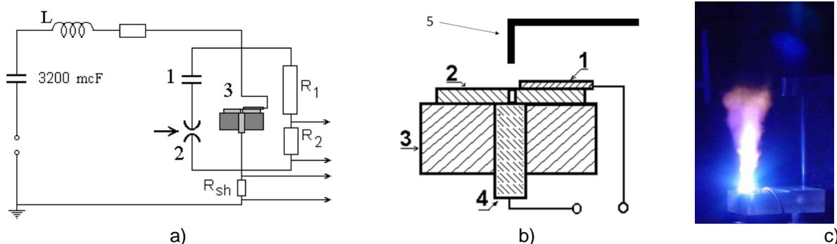
**Fig. 5. Capillary plasma generator. a) 1 – initiating capacity, 2-commutator, 3 –capillary, R<sub>1</sub>, R<sub>2</sub> – resistances of a voltage divider. b) 1,4-electrodes, 2-dielectric plate, 3-plasma generator's base, 5-metallic wire. c) Capillary discharge at organic glass base [3].**
